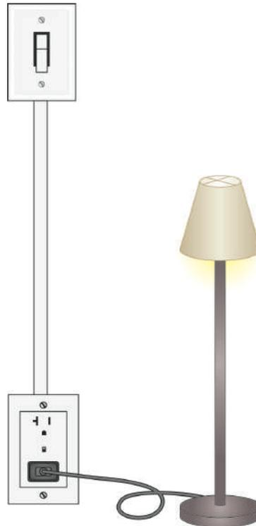
Where a switch controls a receptacle load
