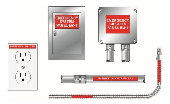
Receptacles that are fed from emergency system required to be identified by a "distinctive color or marking" on the receptacle cover plates or the receptacle.
