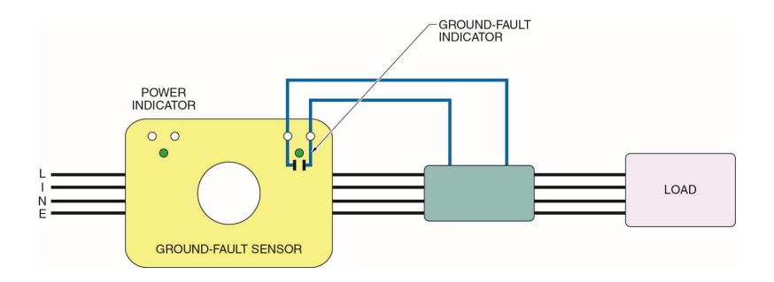
This could lead to nuisance tripping so code language was added at 701.6(D) to clarify that the ground fault sensor can be located at an alternate location for systems with multiple emergency sources connected to a paralleling bus
