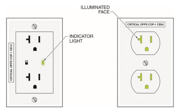
2017 requirement for nonlocking-type, 125-volt, 15- and 20-ampere receptacles supplied from the COPS to have a <u>illuminated face or an indicator light</u> to indicate that power is supplied to the receptacle
