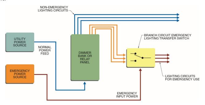
**Definition:** Branch Circuit Emergency Lighting Transfer Switch. A device connected on the land side of a branch circuit overcurrent protective device that transfers only emergency lighting loads from the normal supply to an emergency supply.
