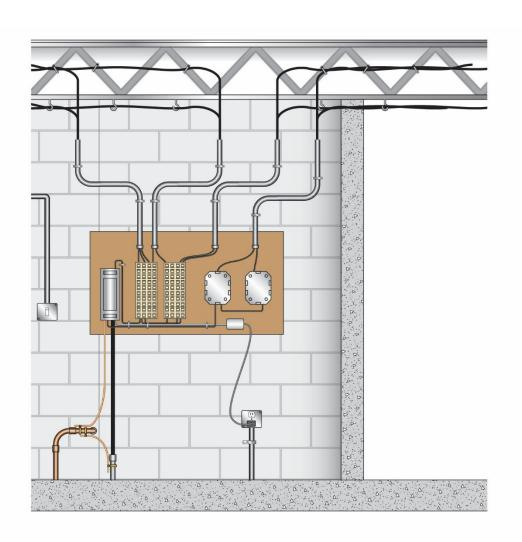
Metallic conduit containing optical fiber entrance cable shall be tied to a grounding electrode by a bonding or grounding electrode conductor per 770.100(B)
