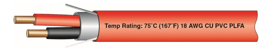
New marking requirements were added for fire alarm circuits requiring a temperature rating to be marked on the jacket of NPLFA and PLFA cables that have a temperature rating exceeding 60°C (140°F) and cable jacket must also show conductor size as well
