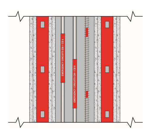
Fire protection provisions for emergency system feeders required for the following occupancies:
