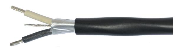
This new exception in 727.4(G) Ex to (5) allows ITC-ER cable to transition between cable trays and between cable trays and utilization equipment or devices for a distance not to exceed 1.8 m (6 ft) without continuous support where not subject to physical damage
